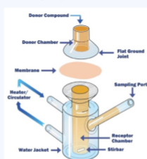
Figure 4. General Franz diffusion cell set-up.
